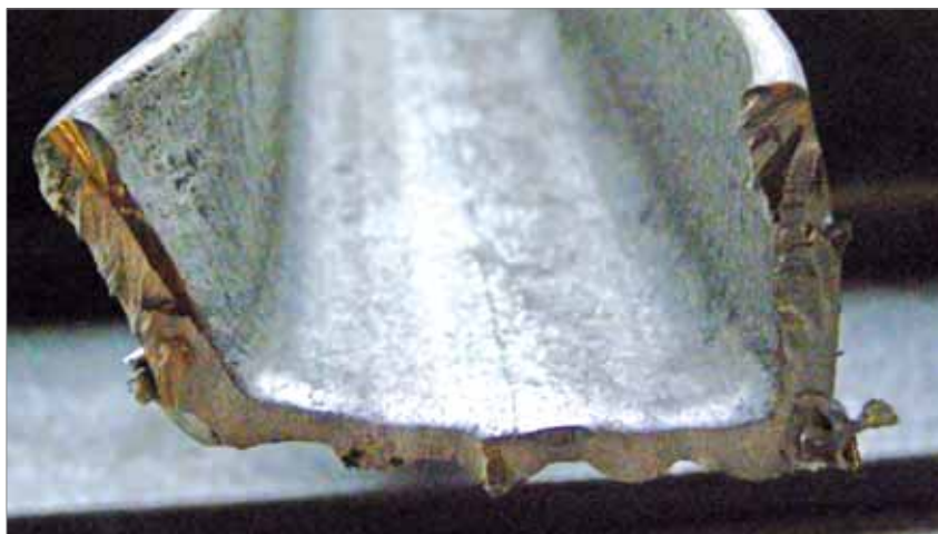
Lom pri strihaní profilu U technológiou CORE.
